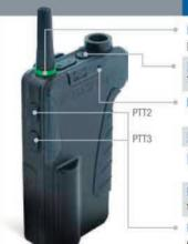
$\begin{tabular}{ll} \textbf{Function Indication Ring: Color-coded rings differentiate between workgroups and portable and base transceivers. User installed. \end{tabular}$
